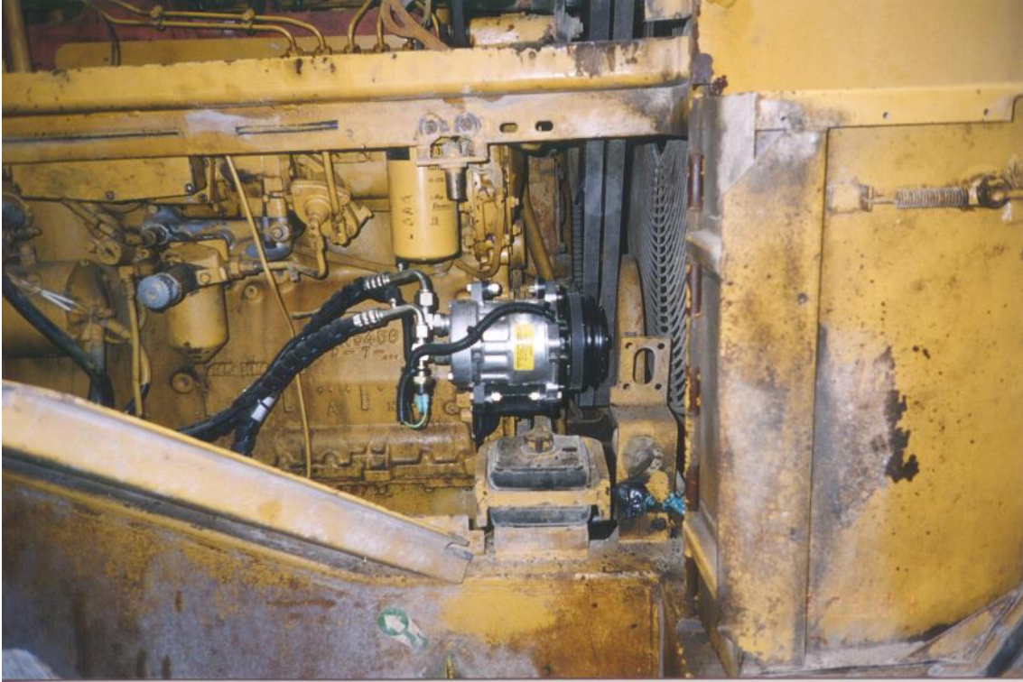
Compressor and mount in place.
