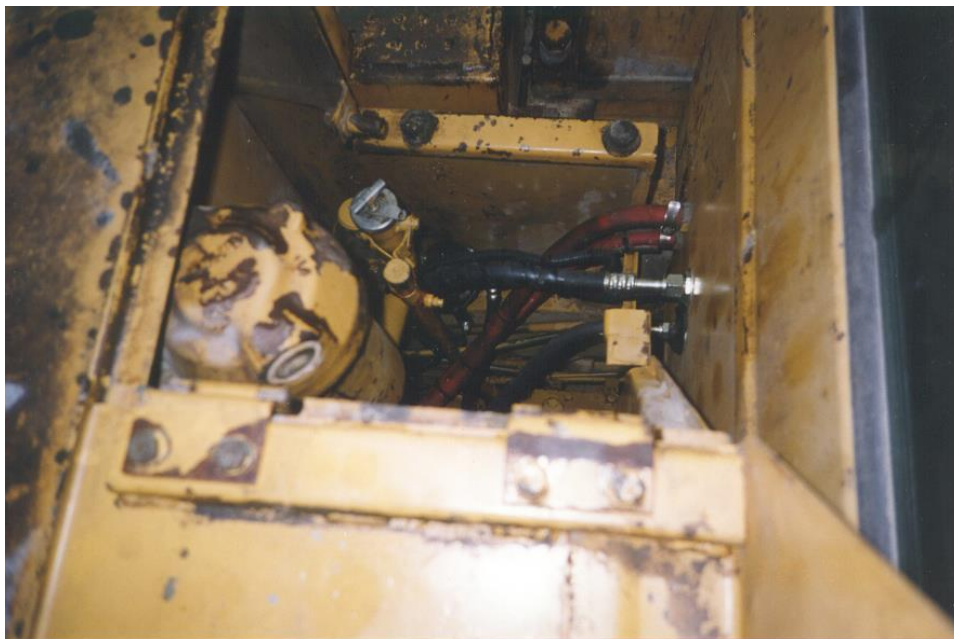
Drier in place with hoses.
